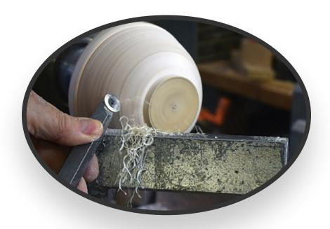
Making a shear scrape is a technique that you can accomplish with steel and carbide tools.
