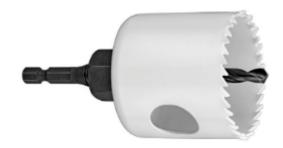
A bi-metal hole saw cuts through wood and metal. A hole saw with a carbide edge works on heavier materials such as ceramic tile and masonry. A hole saw with a diamond edge also works on tile and masonry, but cuts faster than carbide models.
