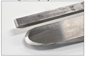
Raising the burr is more critical than the angle of the grind on the end. Use a light touch. Pushing hard raises a bigger burr but it doesn't cut as cleanly. Touch the bevel on the wheel and then raise the handle until you just touch the tip. Feel for the burr.
