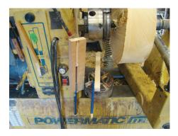
I made the pieces of wood long enough so that as the pencil wears down, the jig will still rest horizontal on the tailstock. I also glued a magnet on the side of the jigs so I can put them on the headstock or at the end of the ways, depending on what I am making. with the jigs attached magnetically to the lathe, they don't fall into the shavings. - Dan Burleson, Troy, MO
