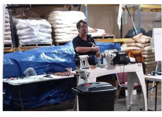
Beaver began his demonstration by illustrating the first cut to a square block of wood. He moved between the lathe and the band saw, showing the various steps needed. He showed his circle-cutting jig, and cautioned folks to take their time, feel comfortable, and - breathe. A microwave was another tool used during his demonstration. This allowed him to steam-fit the thin piece that would extend beyond the bowl.
