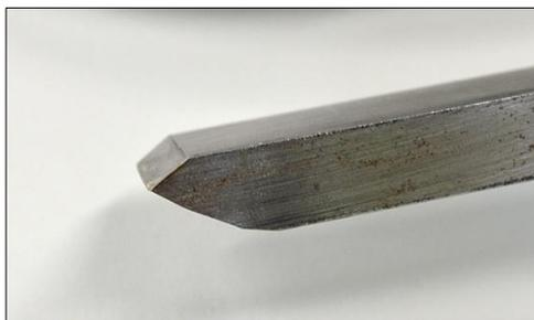
A scraper should be used with a burr raised on the cutting or scraping edge. If the angle between the top surface and the grind or what we will call the bevel is 90 degrees or greater, it won't raise a burr when grinding. Early on I ground all of my scrapers just a little less than 90 degrees.
