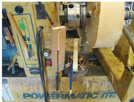
I made the pieces of wood long enough so that as the pencil wears down, the jig will still rest horizontal on the tailstock. I also glued a magnet on the side of the jigs so I can put them on the headstock or at the end of the ways, depending on what I am making. with the jigs attached magnetically to the lathe, they don't fall into the shavings.
