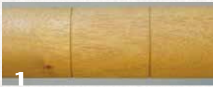
1 Mahogany cylinder prepared with an oval skew chisel. As in all cylinders, the first section on the left will be finished to 320 grit with Method 1 & 2-US. (Note: Methods 1 and 2-US are identical and are referred to as Method 1 & 2-US.) The middle section will be finished to P400 grit with Method 1-EU. The section on the right will be finished with Method 2-EU, which has the extra two grits added (P100 and P150).
