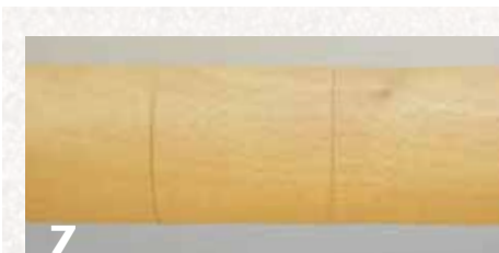
7 Cherry: The left section is finished with Method 1 & 2-US. The middle section is finished with Method 1-EU. The right section is finished with Method 2-EU.
