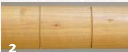
2 Cherry cylinder prepared with an oval skew prior to using any abrasives.
