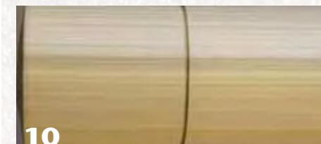
10 Poplar: The apparently smooth finish actually has abrasive scratches, which become noticeable when viewed at an angle, as in Photo 13.
