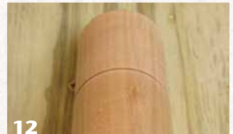
12 Cherry: The abrasive scratches are revealed when the cylinder in Photo 9 is viewed at an angle.
